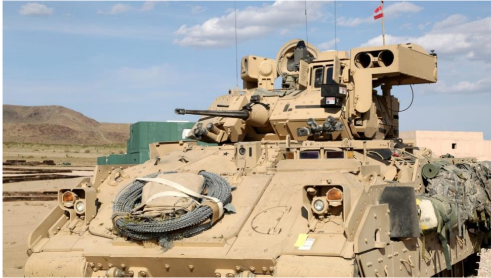
Figure 1: The windows of this Bradley Fighting Vehicle contain high-grade germanium, one of many sources of that could be recycled for reuse.
